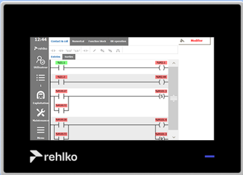
Ladder function for control customization
